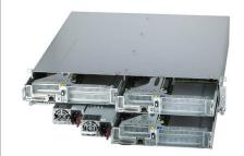
The SYS-211SE-31A balances density (3 nodes) and expandability in a 2U short-depth design, making it an excellent choice for both edge and micro data centers. It provides a flexible platform for compute- and storage-intensive applications, with ample memory capacity and support for enterprise-class NVMe drives.
